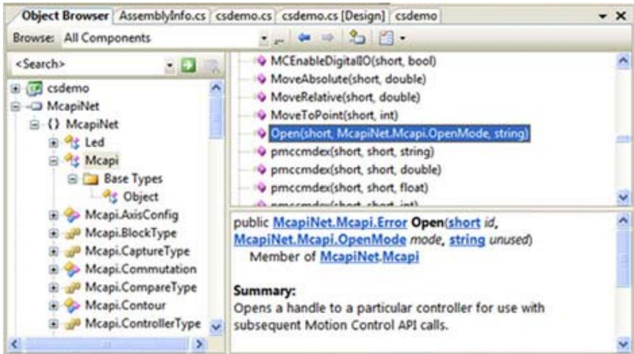
All the programming constants of the MCAPI function library have been migrated to .NET enumerations. McapiNet methods require the use of the correct enumeration types. This makes it almost impossible to pass a bad value for a constant to a McapiNet method in your program. The Open() method for instance will only accept a Mcapi.OpenMode value for the open mode, Visual Studio will consider any other value a compile time error.
