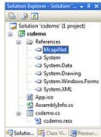
McapNet contains two main classes. The Mcaপি class implements the Motion Control API functions as methods, while the Mcdlg class implements the Motion Dialogs (motor setup dialog, select controller dialog, etc.) as methods. In addition to these main classes there are numerous smaller objects and enumerations that facilitate using McaপিNet in a typesafe object-oriented manner.
