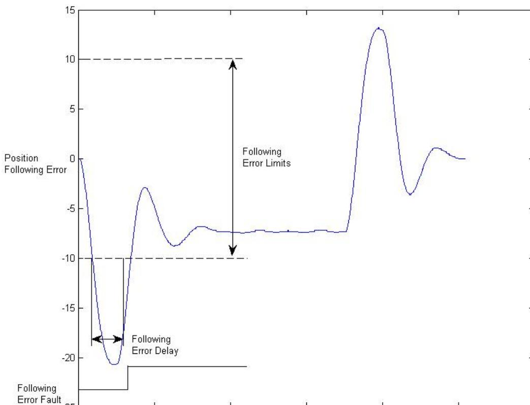
During rapid acceleration and deceleration, the error may easily exceed the desired maximum value and settle within it during constant velocity. In many applications, this is completely acceptable behavior.
